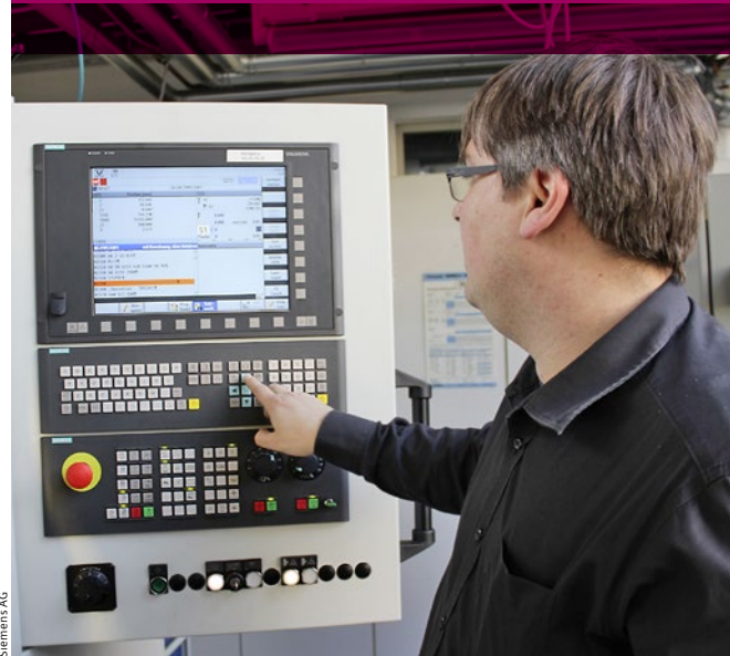
University lecturer Stefan Hirsch transfers CAD/CAM data to the Sinumerik CNC
